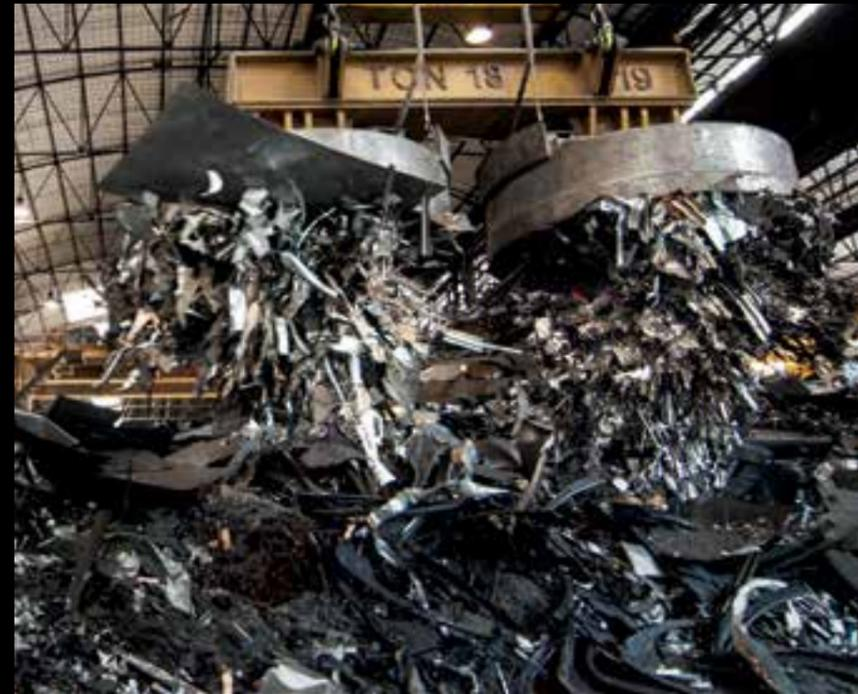
The use of EAF furnaces instead of blast furnaces allows the use of ferrous scrap as raw material, giving an infinite life cycle to steel products that will become scrap and thus raw material again.
